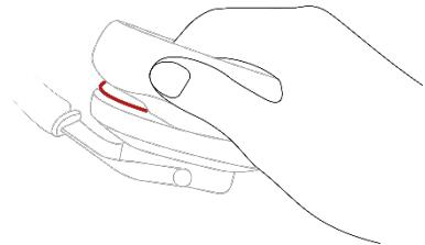
4. Tighten the screws and carefully push the inner plate downwards to lock the cushions into position. Then insert the new foam inlays.
