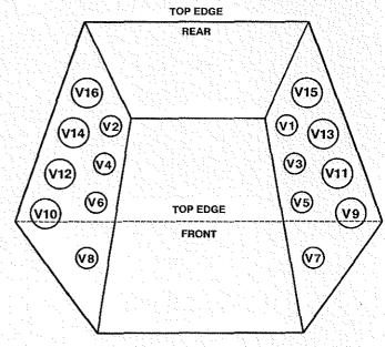
Diagram indicates relative positions of all (16) tubes located on two circuit boards as viewed from the front and looking down from above the amplifier.
