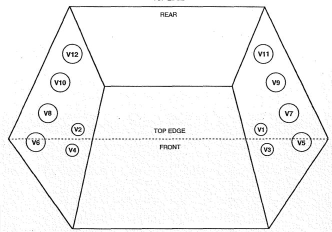
RELATIVE POSITIONS OF ALL (12) TUBES LOCATED ON TWO CIRCUIT BOARDS AS VIEWED FROM THE FRONT AND LOOKING DOWN FROM ABOVE THE AMPLIFIER.
