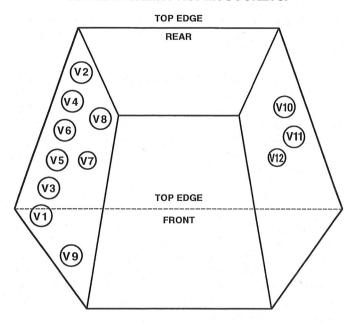
Diagram indicates relative positions of all (12) tubes located on two circuit boards as viewed from the front and looking down from above the amplifier.
