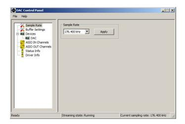
The Mac OS does not allow change of the Sample Rate by the hardware ASIO driver. With the Mac the AUDIO MIDI SETUP Utility has control over the sample rate sent to the Reference DAC. Remember, the Reference DAC defaults to Native mode so it will always lock on and indicate whatever sample rate is being sent by the computer. See the Mac installation instructions for details.
