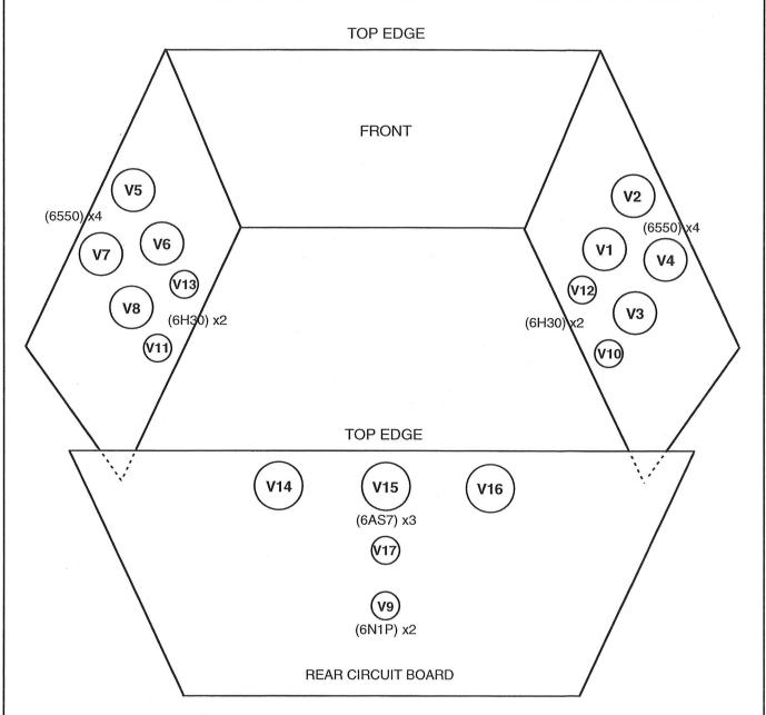
RELATIVE POSITIONS OF ALL (17) TUBES LOCATED ON THREE CIRCUIT BOARDS AS VIEWED FROM THE REAR AND LOOKING DOWN FROM ABOVE THE AMPLIFIER.
