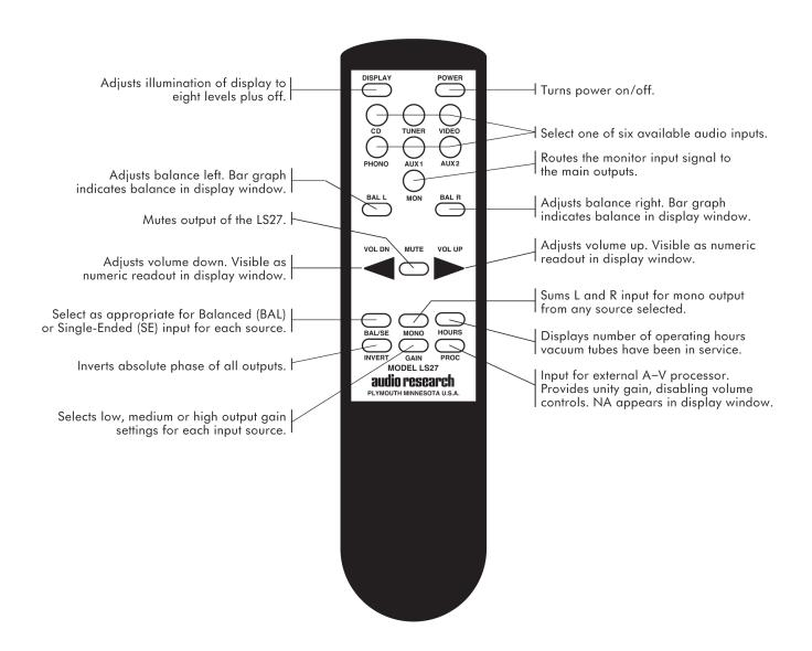
**Note:** All LS27 functions are available on the LS27R hand held remote controller. All functions are indicated in the display window as they are selected. See 'Description of Controls' in this manual for more information.
