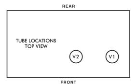
Diagram indicates relative positions of two 6H30 tubes located on circuit board as viewed from the front and looking down from above the preamplifier.
