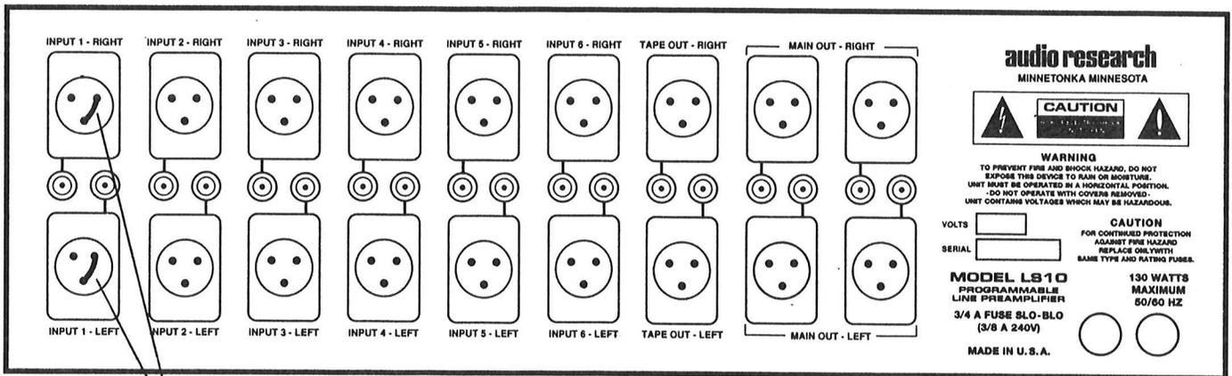
**Note:** Install supplied "U"-shaped shorting jumpers between pins 1 and 3 as shown on the unused XLR input connector pair when making single-ended (RCA) connections to the same input.
