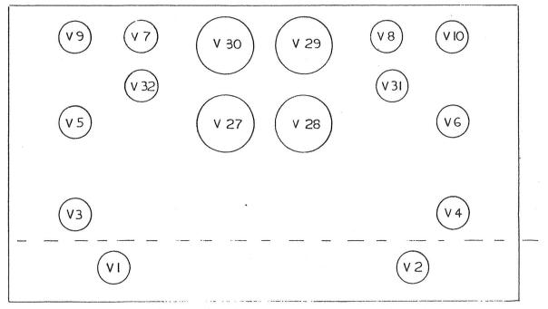
NOTE THAT VI AND V2 ARE BELOW THE CHASSIS - REMOVE BOTTOM COVER FOR ACCESS
