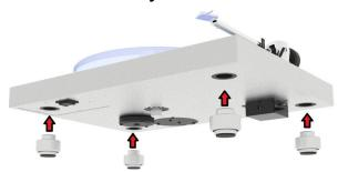
Remove the three feet (5) from the grey foam insert which holds the turntable chassis. Carefully lift the turntable and screw the feet into the thread inserts on the bottom of the turntable. Balance the turntable by using a spirit level before next steps.
